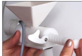
Lift white latch and remove plastic screw. Brush away salt.
