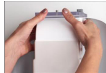
2. Remove the fan by placing your thumbs against the acrylic plate for support, then gently pull the fan while holding the sides.
