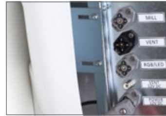
1. Disconnect the plugs of the fan and mill from the electrical box inside the generator.
