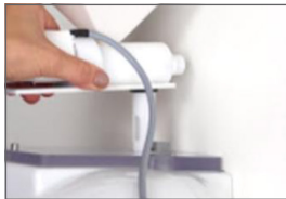
Turn so that hole in tube is facing operator. Empty feeder.
